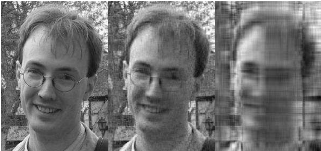
Figure 4: Left: full resolution image (albeit JPEG-compressed). Middle: 16% of the singular values. Right: 4% of the singular values.
